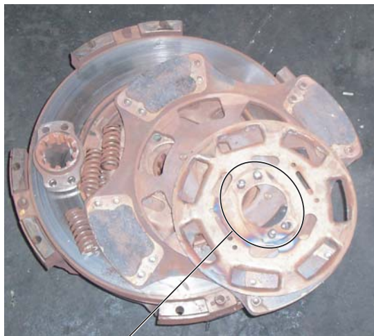
Broken Hub Rivets
