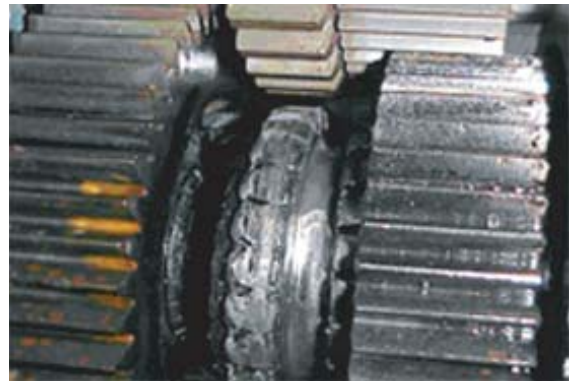
Figure 3: Shift yoke burned and broken off from M/S being skewed.
