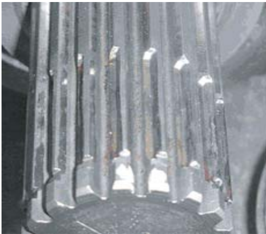
Figure 4: Fretting damage to end of front box mainshaft.
