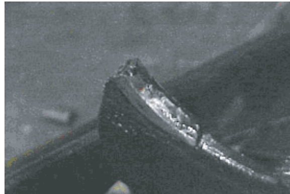
Figure 3: Shift yoke burned and broken off from M/S being skewed.
