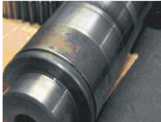
Figure 2: Fretting damage (wear) on countershaft from a loose gear.
