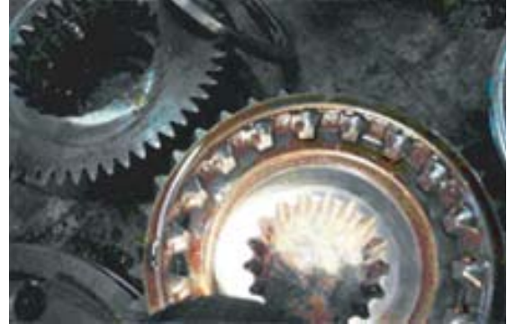
Figure 1: Fretting damage on the auxiliary drive gear clutching teeth.
