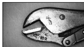
Upper Teeth Worn/Missing
