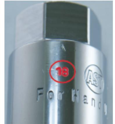
Sockets marked "For Hand Use Only", will not be warranted if damaged by use with a Power/Impact Tool.
